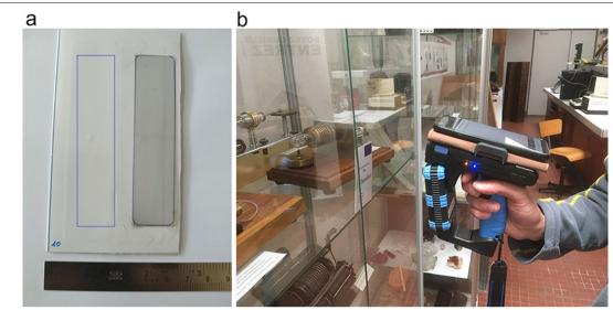
Fig. 1 a RFID corrosion sensor. b interrogation of the sensor by a commercial RFID reader
