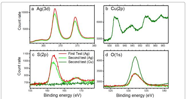
Fig. 3 XPS spectra of the sensitive parts (silver and copper) of the RFID sensors after the two exposure tests in the storage room. a Ag(3d), b Cu(2p), c S(2p) and d O(1 s) spectra
